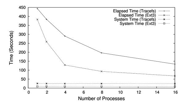
Figure 4.5: Elapsed and system times for Postmark with Ext3 and Tracefs with multiple processes
