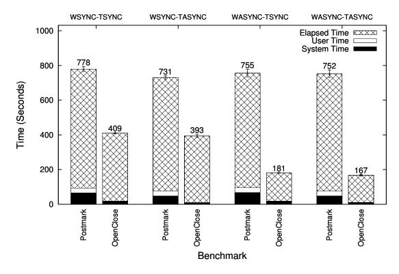
Figure 4.4: Execution times for Postmark and OpenClose. Bars show system, user, and elapsed times for all combinations of asynchronous filter and trace file writes.
