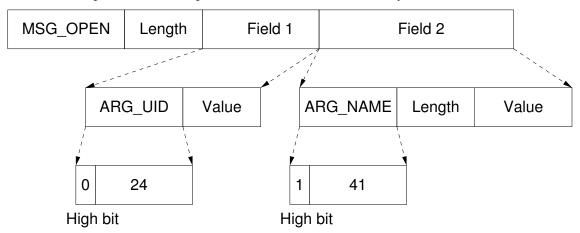
Figure 2.5: An example of a trace message. Each message contains a message identifier, a length field, and multiple arguments. The highest bit of the argument identifier indicates that the argument has a length field.
