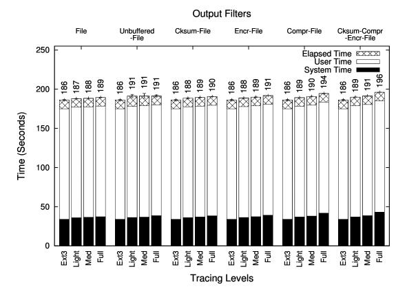
Figure 4.1: Execution times for an Am-Utils build. Each group of bars represents an output filter configuration under LIGHT, MEDIUM, and FULL tracing. The leftmost bar in each group shows the execution time for Ext3.
