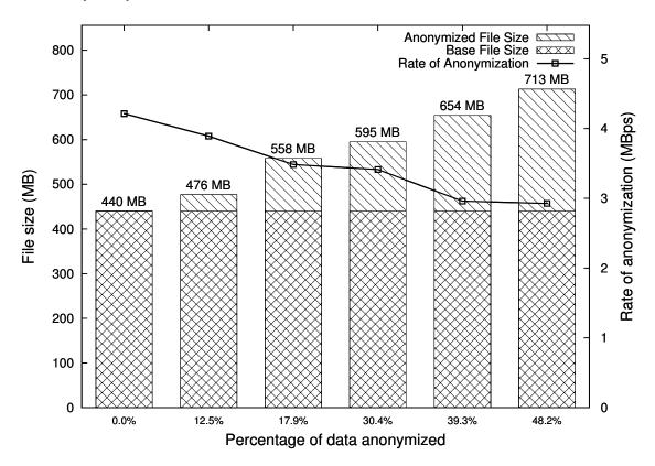
Figure 4.6: Trace file anonymization rates and increase in file sizes for different portions of traces anonymized. The  $Y_1$  axis shows the scale for file sizes whereas the  $Y_2$  axis shows the scale for the rate of anonymization.
