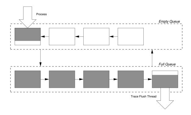
Figure 3.2: The asynchronous filter for performing stream transformations asynchronously. A separate kernel thread is used to transform the stream and write traces to stable storage.
