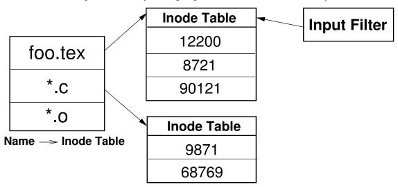
Figure 3.1: The file name cache for tracing based on file names and extensions. The first level table maps a name to an inode number table that stores inode numbers with that name. An input filter has a direct reference to the inode number table.
