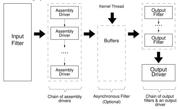
Figure 2.2: Architecture for a Tracefs tracer. Assembly drivers generate a trace stream that is transformed by output filters before being written out by an output driver. An optional asynchronous filter buffers the trace stream that is processed by a separate kernel thread.
