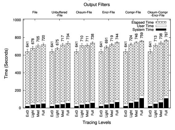
Figure 4.2: Execution times for Postmark. Each group of bars represents an output filter configuration under LIGHT, MEDIUM, and FULL tracing. The leftmost bar in each group shows execution times for Ext3.
