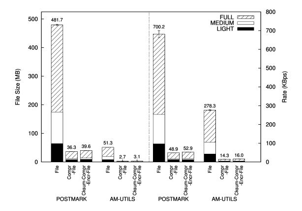
Figure 4.3: Trace file sizes and creation rates for Postmark and Am-Utils benchmarks. Each bar shows values for FULL, MEDIUM, and LIGHT tracing. The left half depicts file sizes and the right half depicts trace file creation rates
