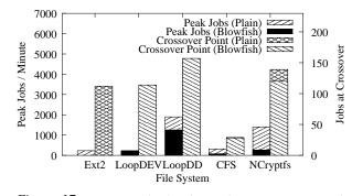
Figure 17: AIM7 results for the workstation. Note: Peak jobs/minute is using the left bars and scale. Crossover is using the right bars and scale.
