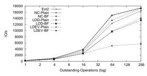
Figure 16: PGMeter: File server I/O operations per second
