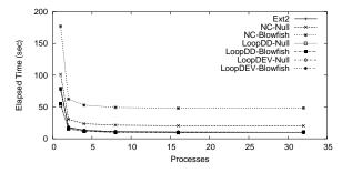
Figure 14: PostMark: File server elapsed time with two CPUs
