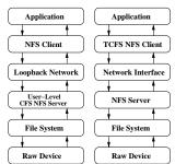
Figure 2: Call path of network-based systems. CFS is on the left, TCFS is on the right.
