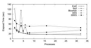
Figure 7: PostMark: LOOPDD elapsed time for the workstation. Note: Null, Blowfish, and AES additionally have points for 1–8 in one process increments rather than exponentially increasing processes.
