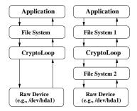
Figure 1: Cryptoloop stacked on top of a raw device (left) and a file (right)
