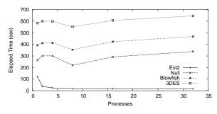
Figure 9: PostMark: CFS elapsed time for the workstation
