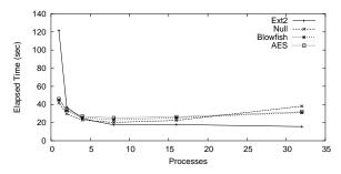
Figure 8: PostMark: LOOPDEV elapsed time for the workstation, with  $nfract_sync = 90\%$ . Note: 3DES is not included because it does not display this anomaly.
