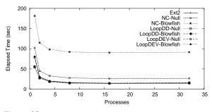
Figure 13: PostMark: File server elapsed time with one CPU
